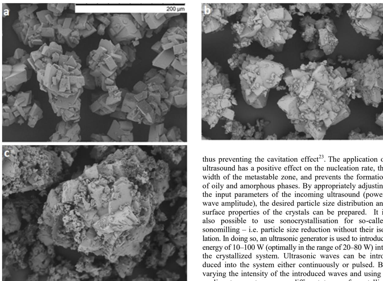
Fig. 4. SEM images of crystalline APIs monitoring the effect of the grafting material on the final crystal. a) API grafted with sieved material, parameter D90 = 42  $\mu\text{m}$ ; b) API grafted with the material in a), parameter D90 = 88  $\mu\text{m}$ ; c) API grafted with the material in b), parameter D90 = 102  $\mu\text{m}$
