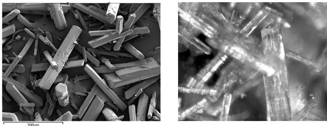
Fig. 8. Comparison of SEM image (left) and microscopic image of the same API obtained with the Blaze system (right)
