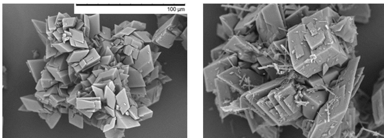
Fig. 9. Comparison of SEM images of crystalline API obtained by grafting material with different specific surface area – SSA (polymorphic form 1, SSA = 2 m<sup>2</sup>/g – left; mixture of polymorphic forms 1 and 2, SSA < 1 m<sup>2</sup>/g – right)
