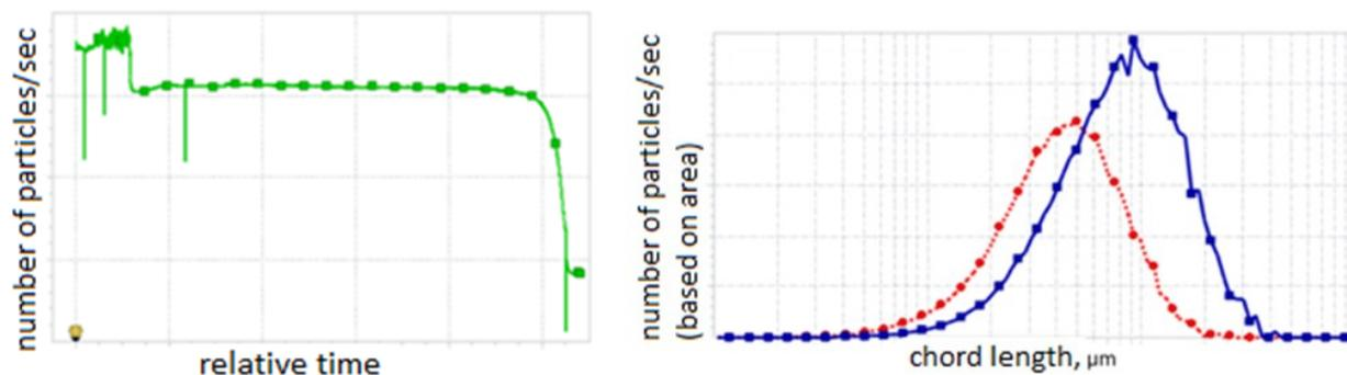
Fig. 6. FBRM record. Sharp decrease in the total number of particles in the crystallizing suspension over time (left), shift in the distribution of particle lengths towards larger particles (right).
