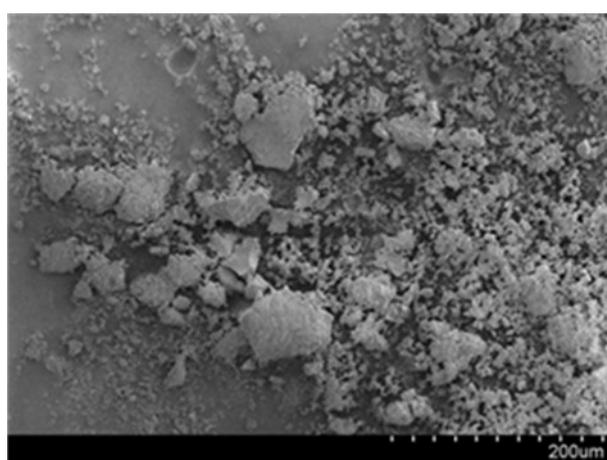
Fig. 3. Left: SEM image of the material called "thermodynamic crystal", obtained at relative supersaturation  $\Delta c = 2$ . Right: SEM image of a material called "kinetic crystal" obtained at relative supersaturation  $\Delta c = 20$
