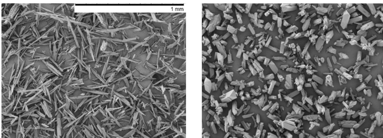
Fig. 7. SEM recording. Dimorphic transformation of one crystal modification (left) to another (right). Electron microscope images confirm the laser probe recording, see Fig. 6 right
