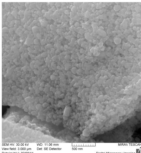
Fig. 1. SEM image of prepared Co metal nanoparticles
